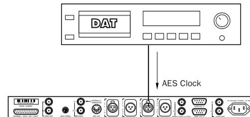
Connecting SYNC I/O to an AES/EBU device
