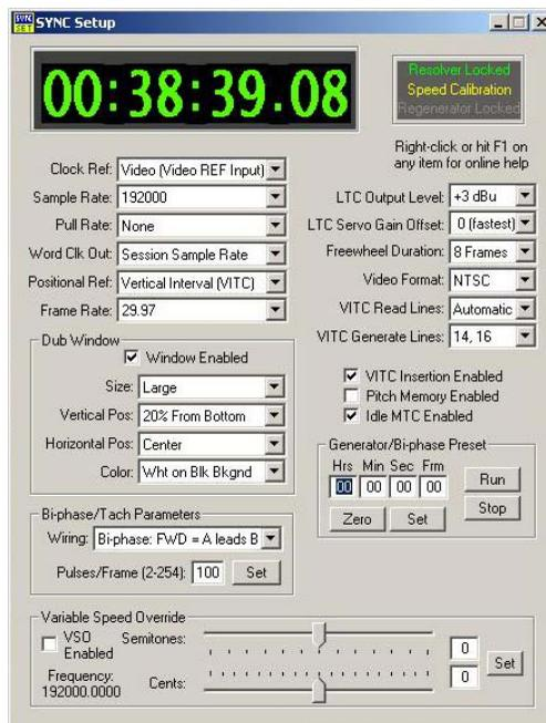
SYNC Setup window (SYNC I/O Setup software utility)
